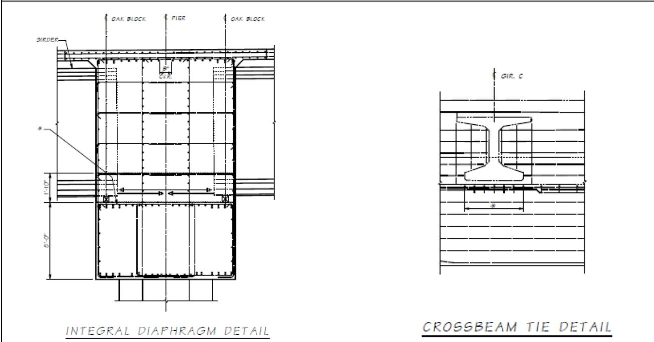
Figure 3: Lower Crossbeam Ties
