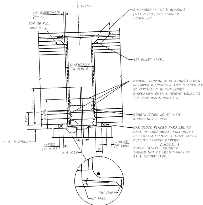
End Type C (Intermediate Hinge Diaphragm)
