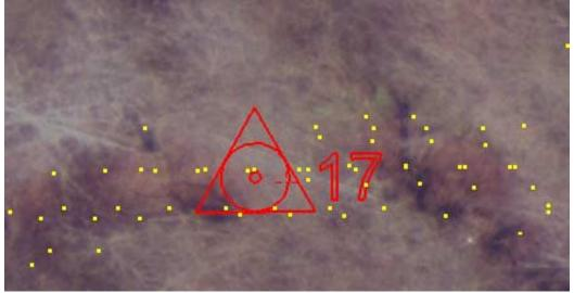
LIDAR vertical differences: +0.34ft. & -0.12ft. LIDAR horizontal point proximity to survey point: .09ft. & .09ft.
