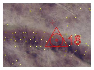
LIDAR vertical differences: +0.45ft. & +1.79ft. LIDAR horizontal point proximity to survey point: 1.18ft. & 8.1ft.
