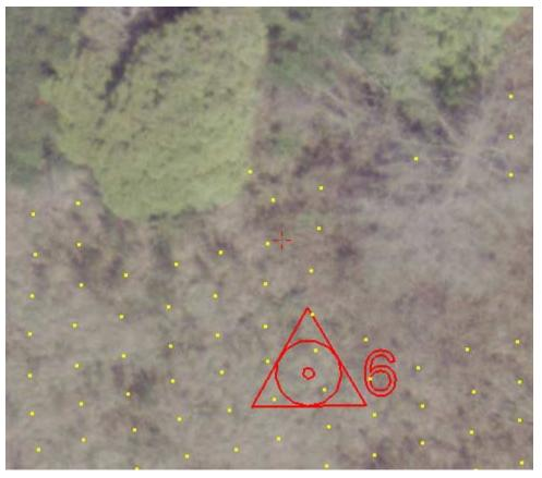
LIDAR vertical differences: +0.97ft. LIDAR horizontal point proximity to survey point: 2.2ft. *QC7*-East side of SR405 on the pavement near a retaining wall. Transportation corridor landscape. Trees and obstructions to the east.
