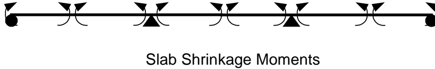
Figure 27 Slab Shrinkage Moments
