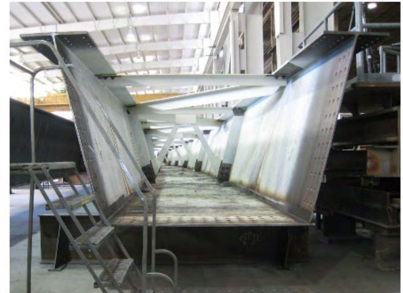
Figure 12.2 Internal Intermediate Cross Frames and Top Flange Lateral Bracing
