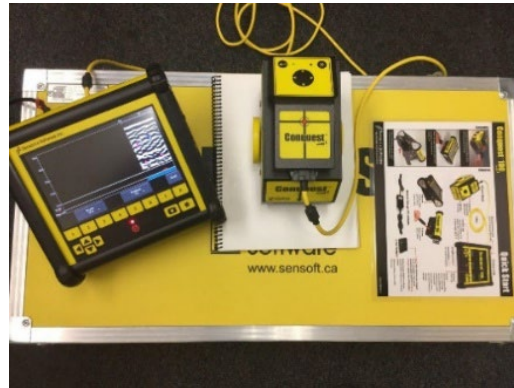
Ground Penetrating Radar (GPR)
