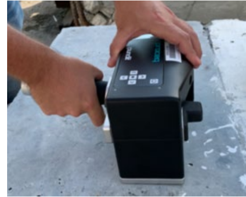
Phased Array Ultrasonic (PAU)
