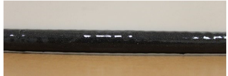
Modification (i) FRP Bar with Iron Particle Coating
