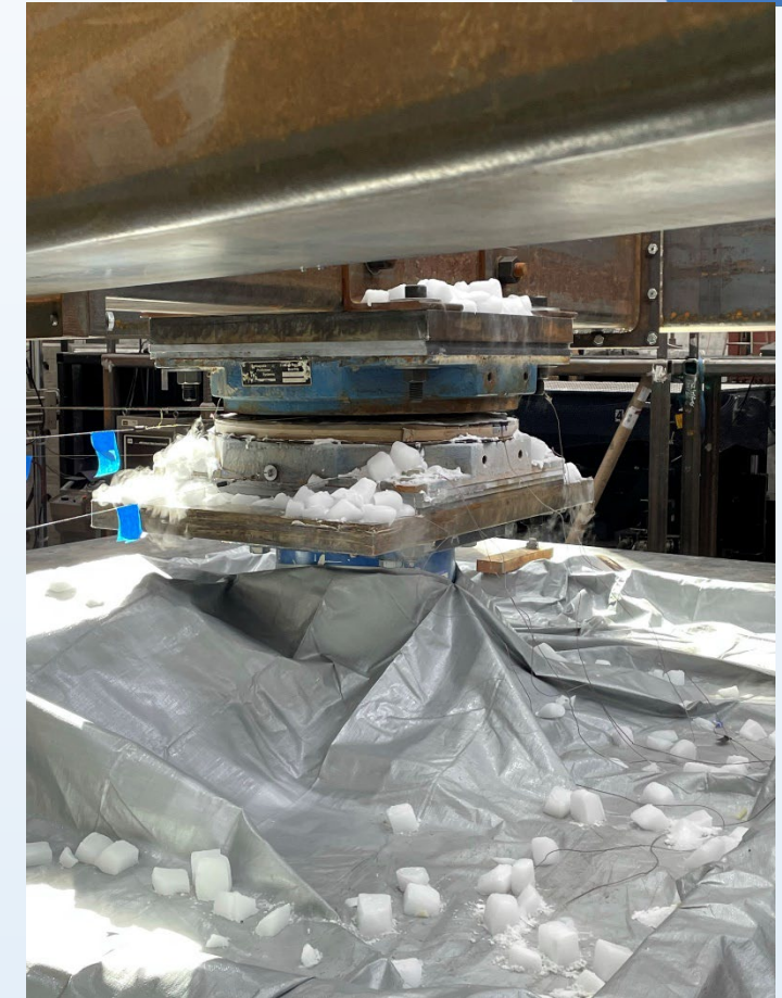
Bearing just prior to “frozen test”; insulation box removed
