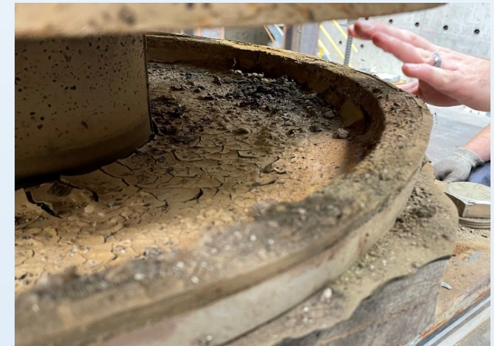
As-received condition of formerly in-service FPS bearing
