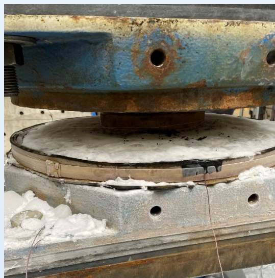
Old Susitna 1 with ice frozen in cavity
