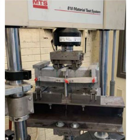
Flexural Prism ASTM C 1609
