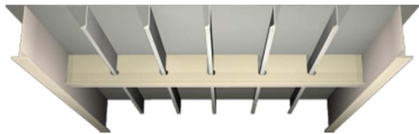
Conventional stiffened steel structure
