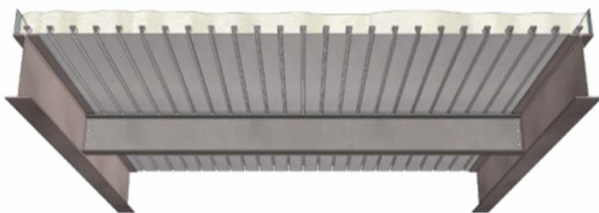
Conventional concrete-steel composite structure
