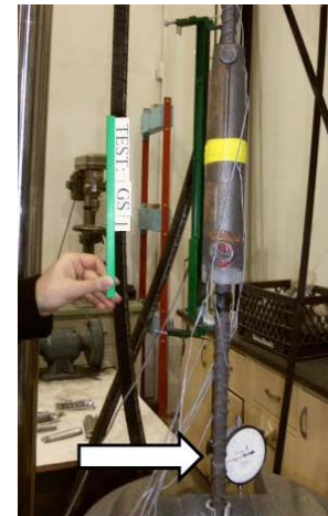
Location of rupture
