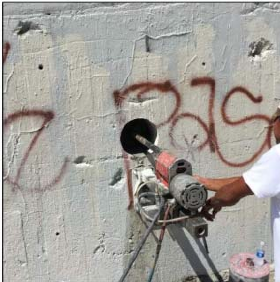
Figure 3 – Coring During the Pier Invasive Investigation
