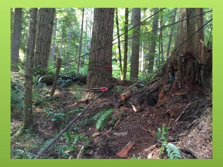
Cable tension approximately 10X payload.
