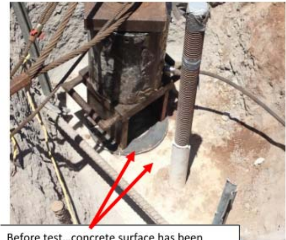
Before test...concrete surface has been ground smooth and new jack chair with plates distribute load to concrete.
