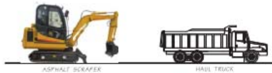
ASPHALT REMOVAL TRAIN
