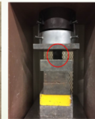
Testing of 2" cube (ASTM C109)
