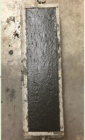
Casting of 3" x 4" x 16" prism flexure specimens
