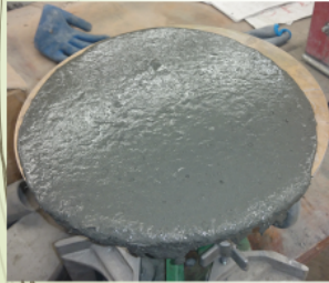
Flow test of UHPC
