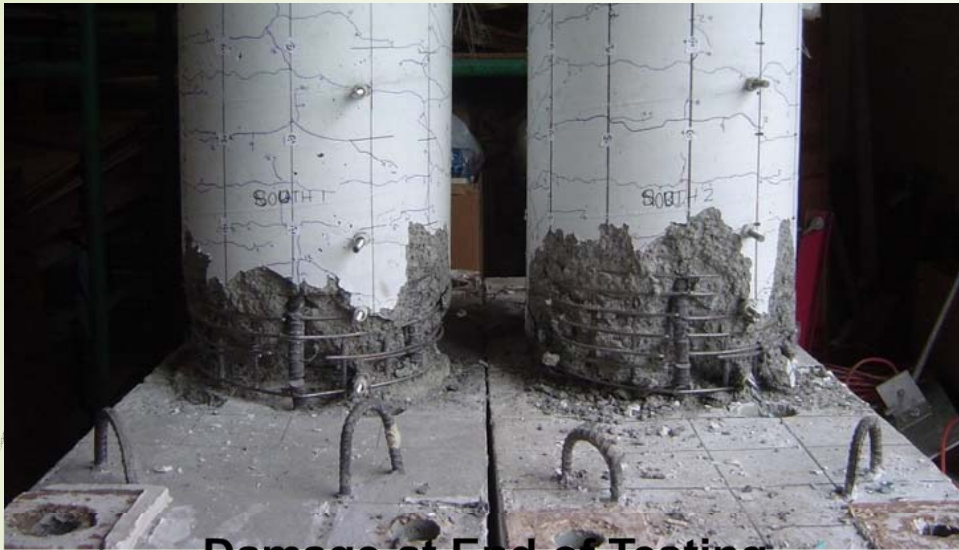
Damage at End of Testing
