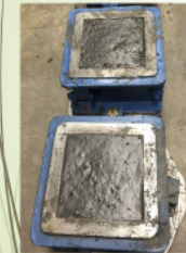
Testing of 4" cube (ASTM C109)
