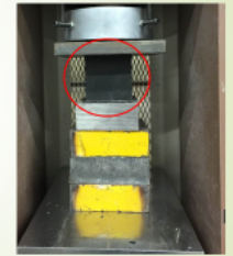
Testing of 2" cube (ASTM C109)
