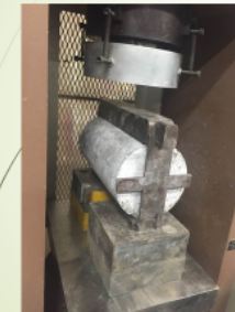
Splitting tensile strength testing
