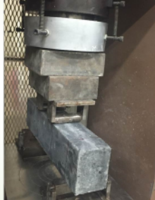
Flexural testing of 3" x 4" x 16" in. specimen (span = 12")
