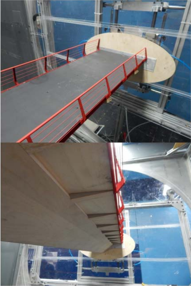
Views of the 1:15 scale sectional model in the wind tunnel
