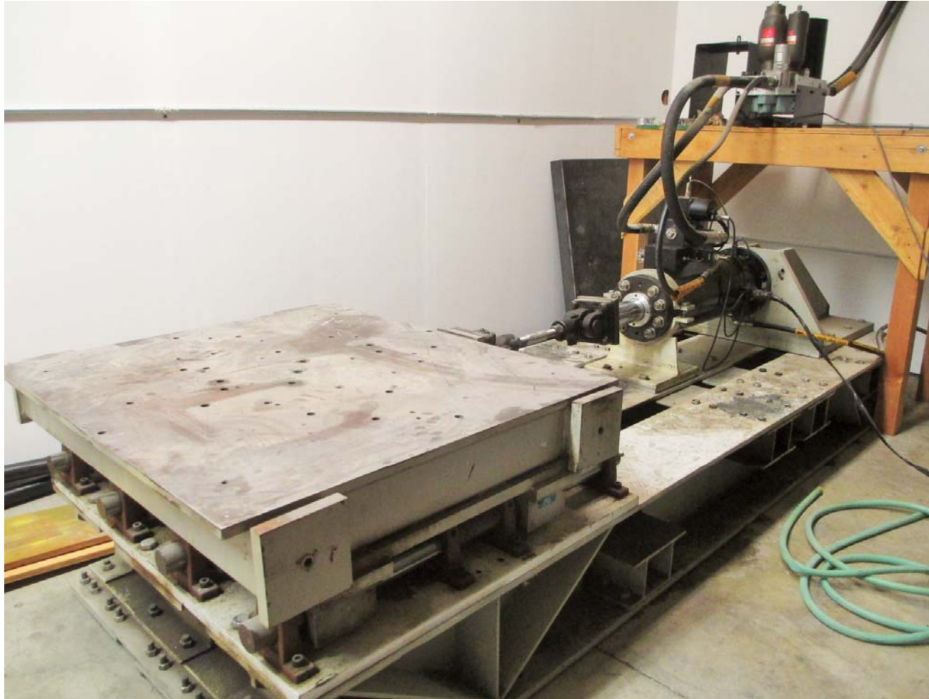
4.5 ft x 4.5 ft hydraulically powered horizontal shake table, 10 kips capacity and \pm 3 in stroke
