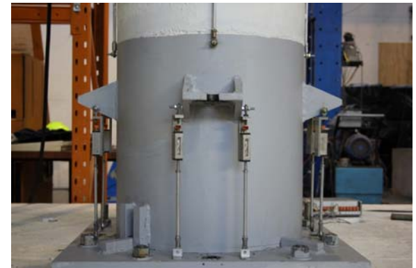
Half-scale bent with DCR connections
