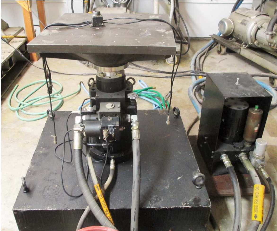
2 ft x 2 ft hydraulically powered vertical shake table, 3 kips capacity
