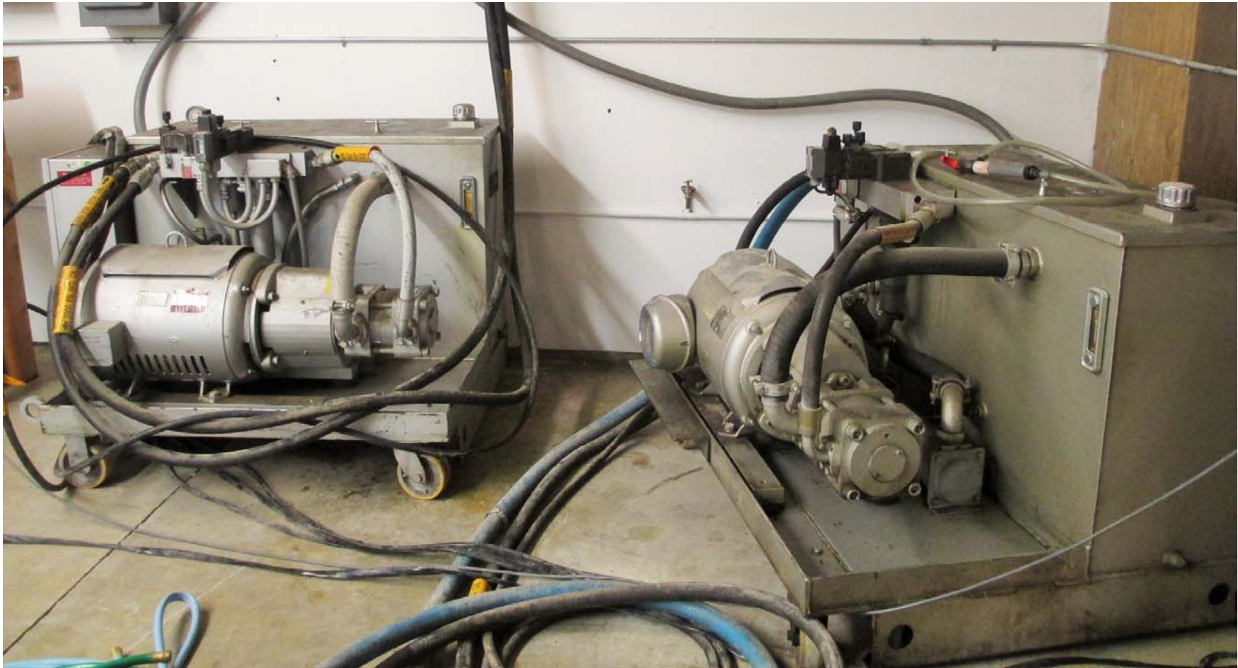
Powerful hydraulic pumps for the shake tables and other actuators
