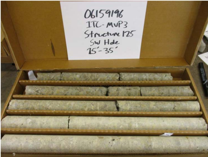
Structure 125 – Southwest Core. Concrete cores from 25 to 35 feet.
