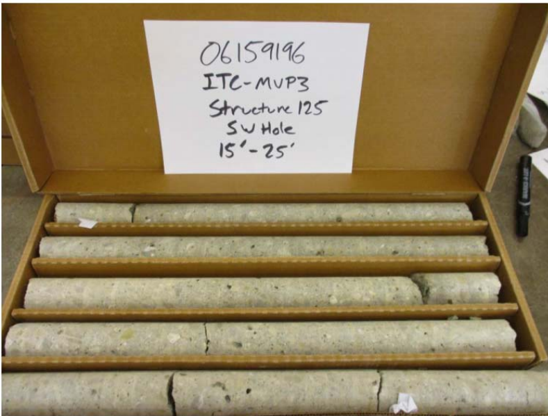
Structure 125 – Southwest Core. Concrete cores from 15 to 25 feet.
