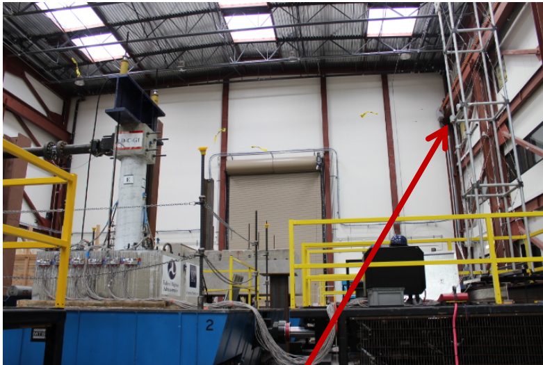
String pots connected to the rigid frame
