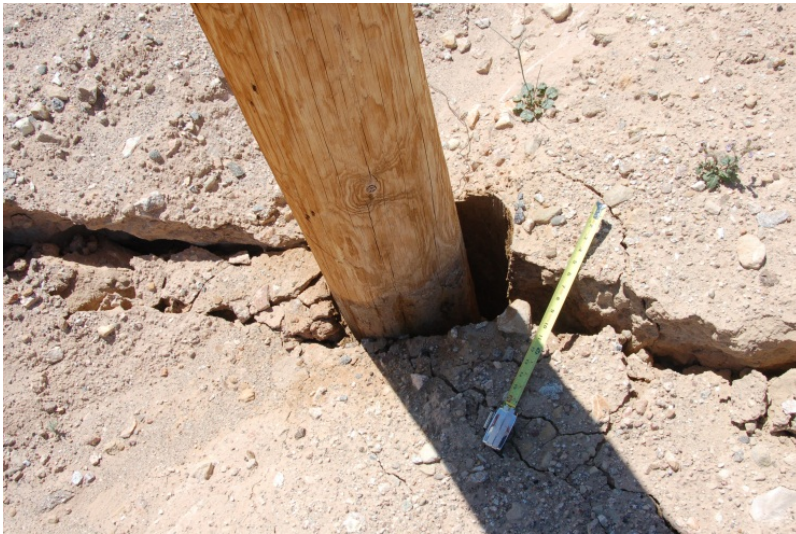
Desirable foundation behavior
