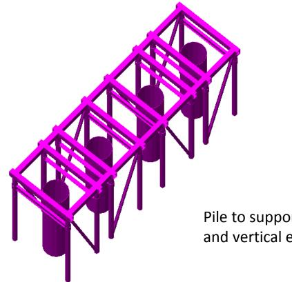
Pile to support oscillator lateral and vertical extraction forces
