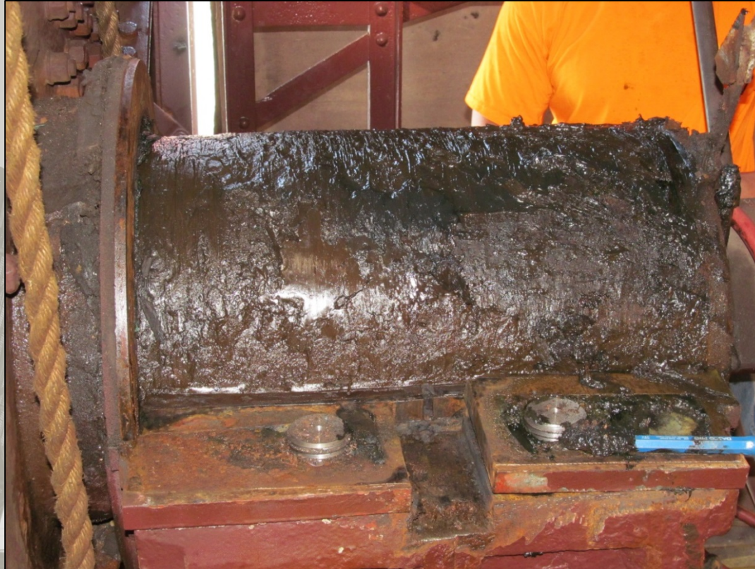
Outboard bearing after cap removal - trunnion journal covered with lubricant
