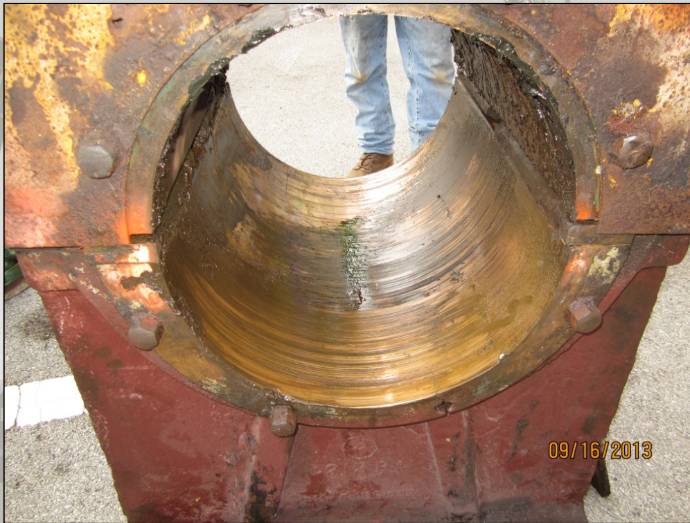
Bearing after removal - Note poor condition of the bearing
