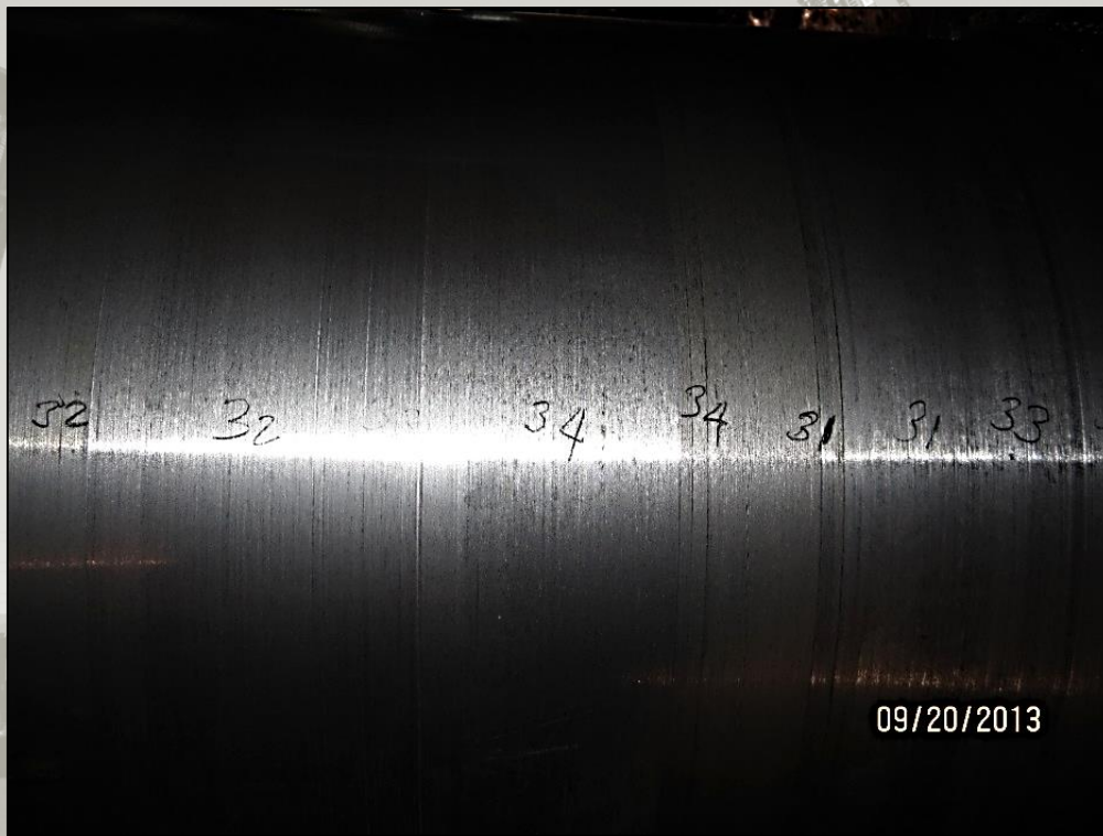
Field machining – Dimensions on shaft
