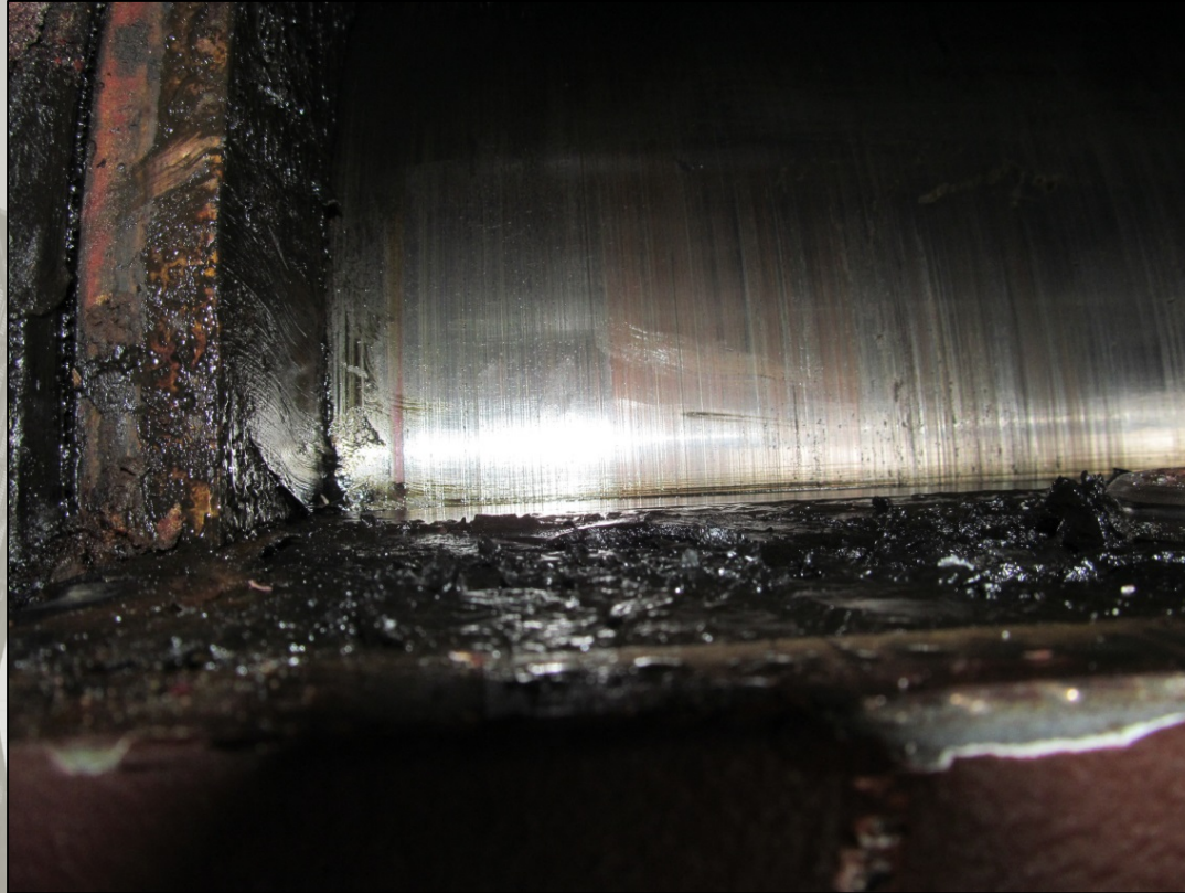
Inboard trunnion journal – close up of inboard end with light scoring and bronze embedment
