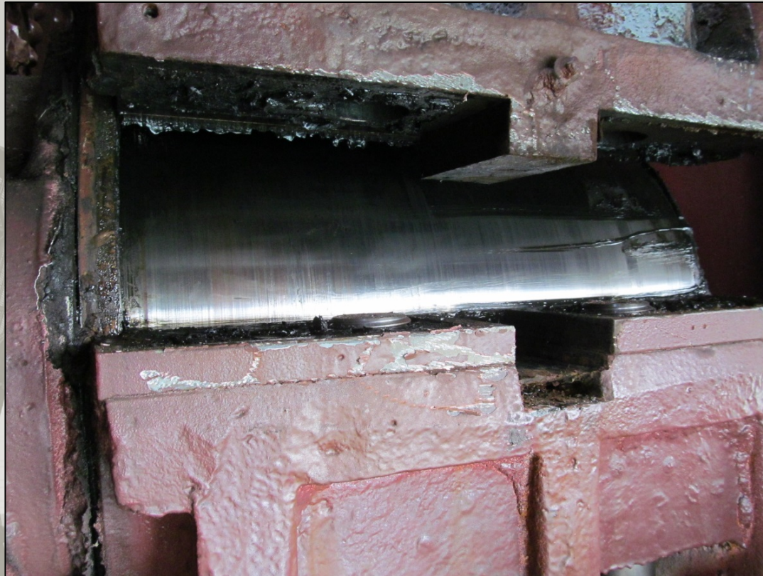
Inboard trunnion journal - generally good to fair condition
