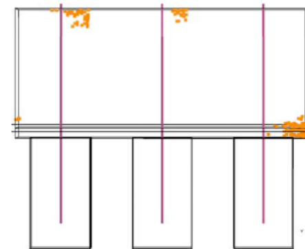
Elevation View: Transverse Loading Tension Zones
