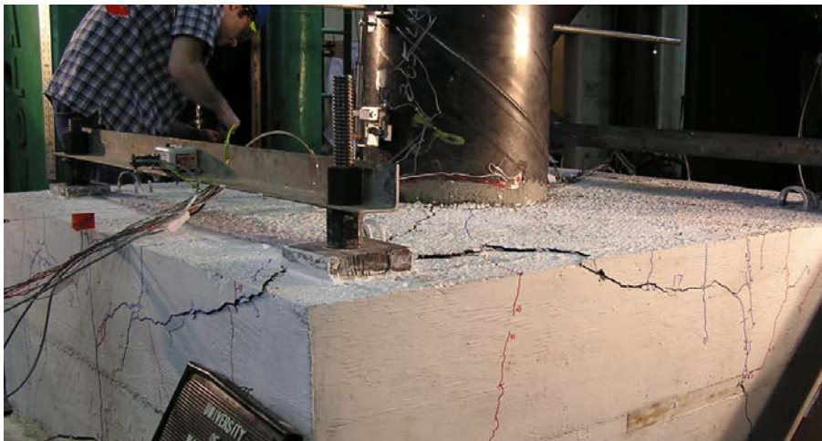
footing uplift: 4% drift
