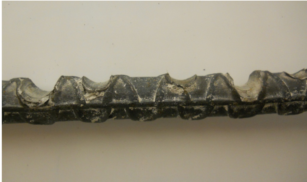
Planer Damage to #5 bar Showing 5/8" tooth spacing
