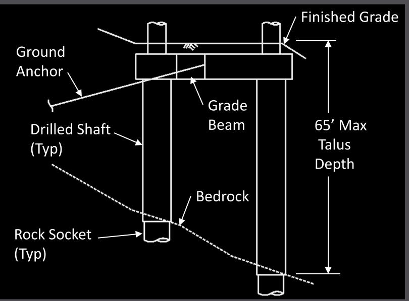
Tensioned Ground Anchors Help Mobilize Landslide Pressure
