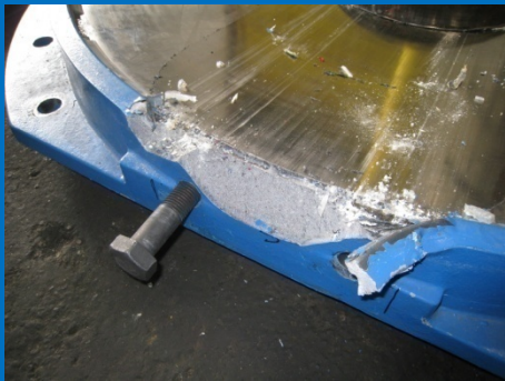
Shear Ring Failure
