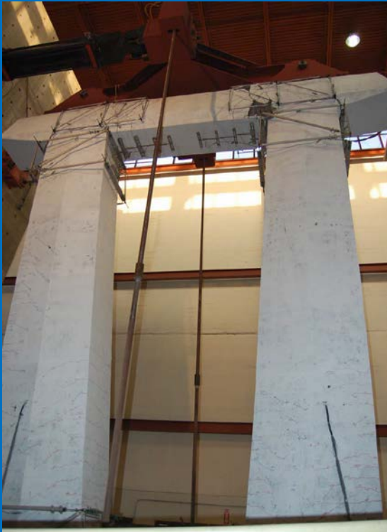
Test Specimen and Cracks \mu = 2
