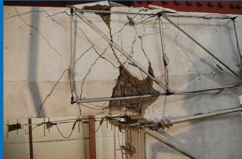
South Column to Cap Beam Joint @ -15" Disp \mu 5
