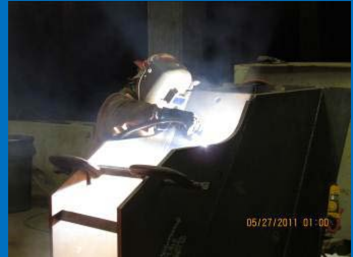
Complicated welding inside the box with 100%UT
