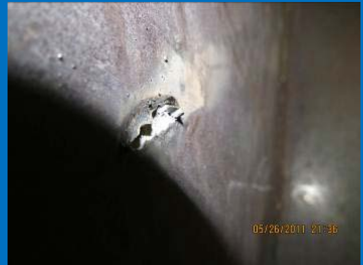
Complicated welding inside the box with 100%UT
