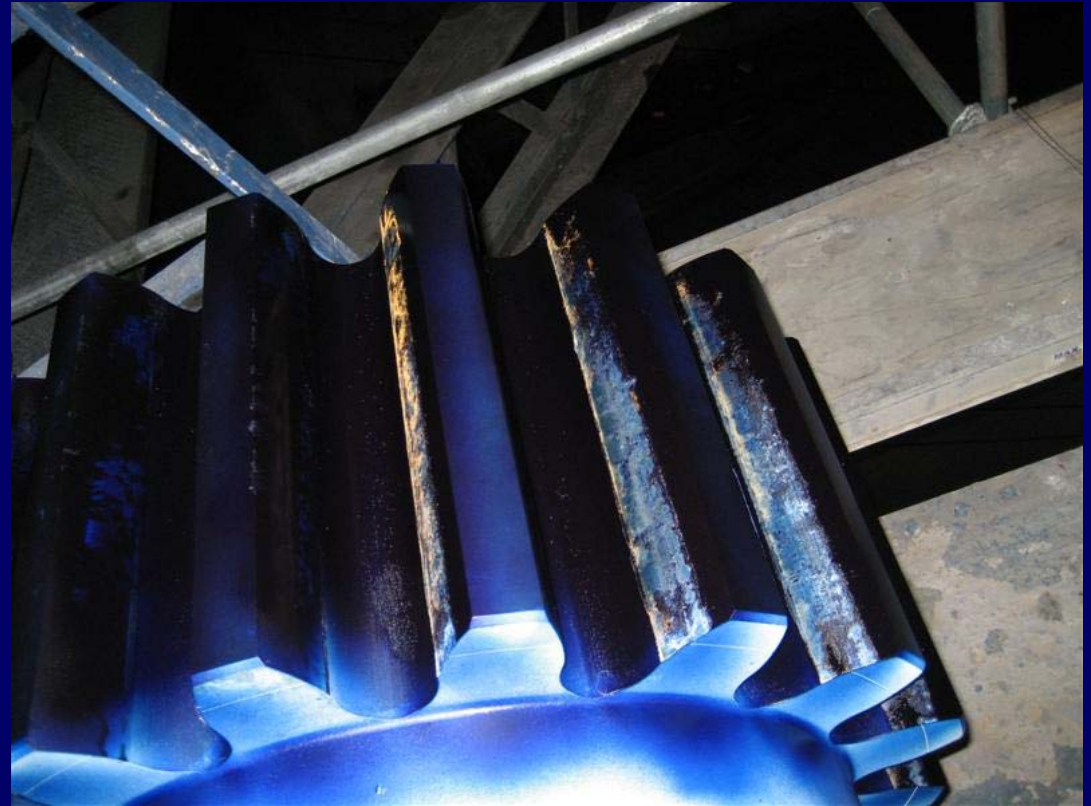
Evaluating Rack Pinion Tooth Contact During Installation Of The Secondary Reducers
