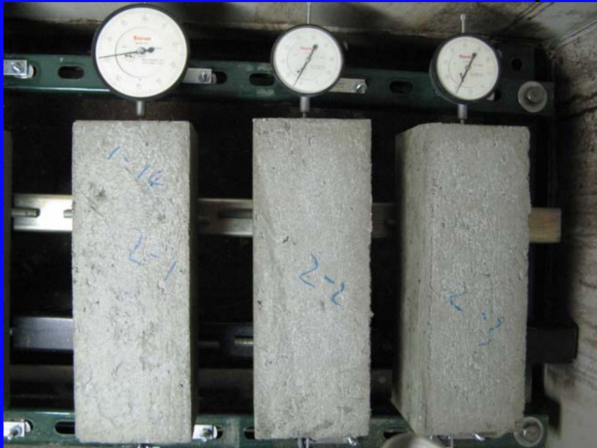
Free Shrinkage Test
