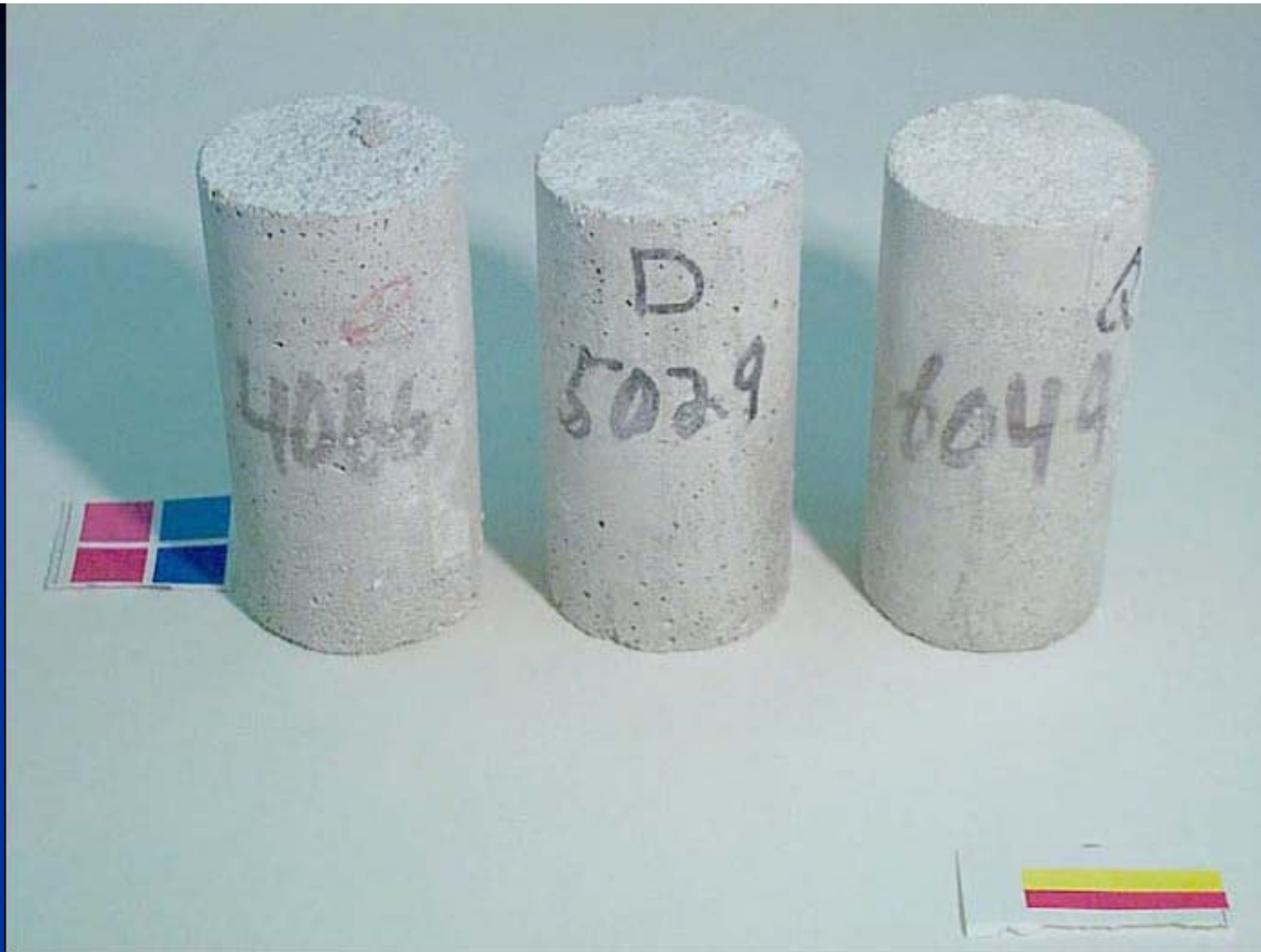
Cylinders (2 in by 4 in) exposed to NaCl solution after 84 days of constant low temperature test. From left to right: 0.40, 0.50, 0.60 w/c ratio
