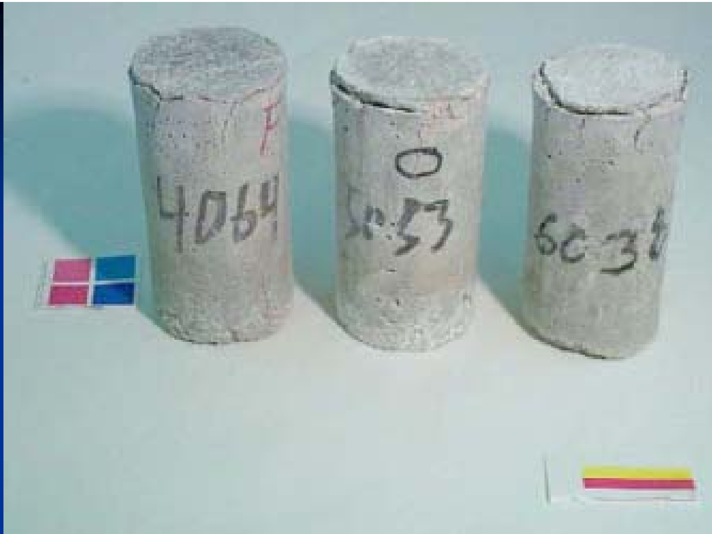
Cylinders (2 in by 4 in) exposed to MgCl_2 solution after 84 days of constant low temperature test. From left to right: 0.40, 0.50, 0.60 w/c ratio
