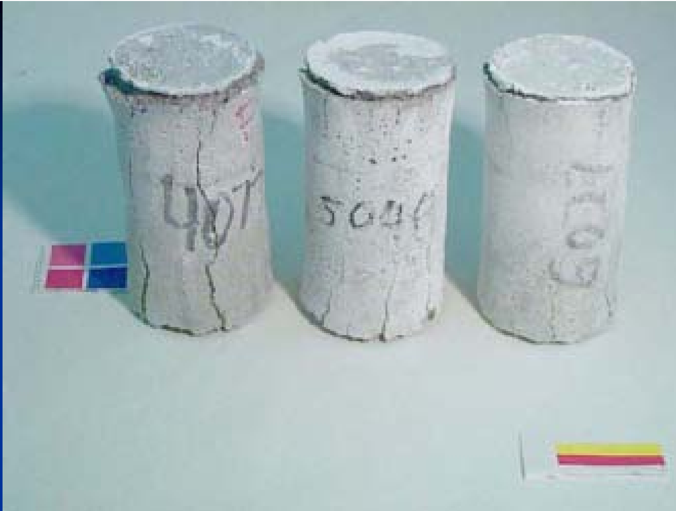
Cylinders (2 in by 4 in) exposed to \text{CaCl}_2 solution after 84 days of constant low temperature test. From left to right: 0.40, 0.50, and 0.60 w/c mortar cylinders.
