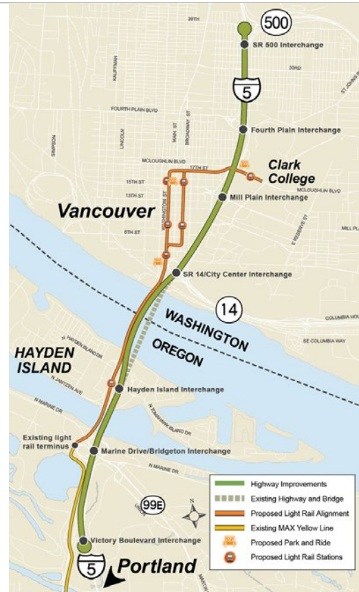
Prior project planning included a light rail transit extension of the Portland MAX system to downtown Vancouver and Clark College.
