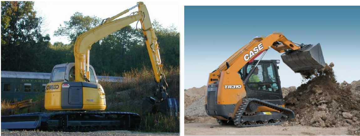
Exhibit 6: Examples of 4-5 psi ground pressure equipment.
