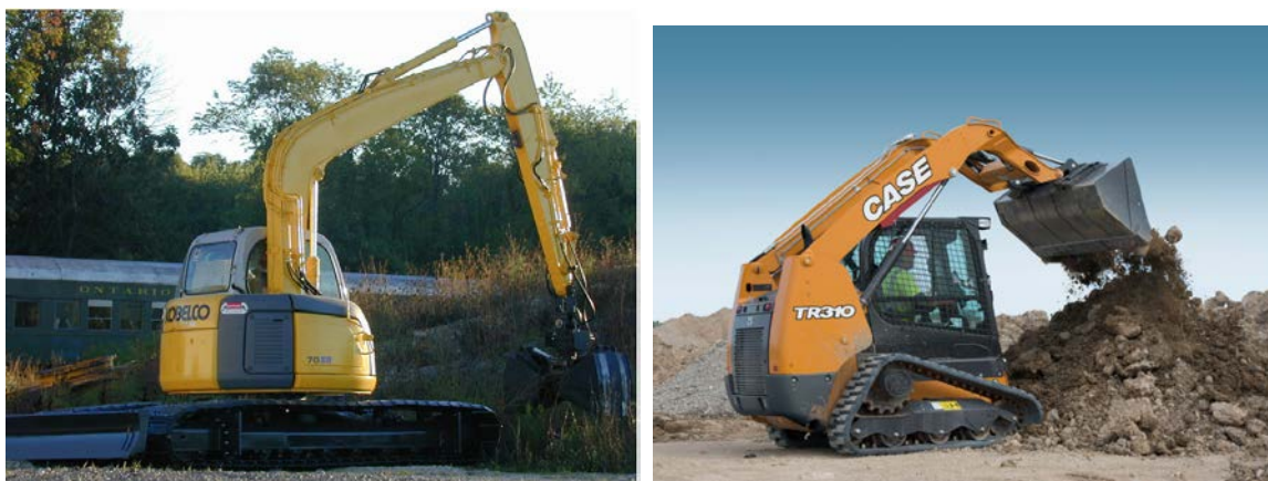
Exhibit 6: Examples of 4-5 psi ground pressure equipment.
