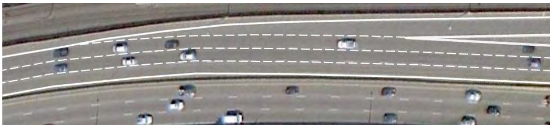
Figure 2 - Typical Freeway Entrance Ramp Merge Area
