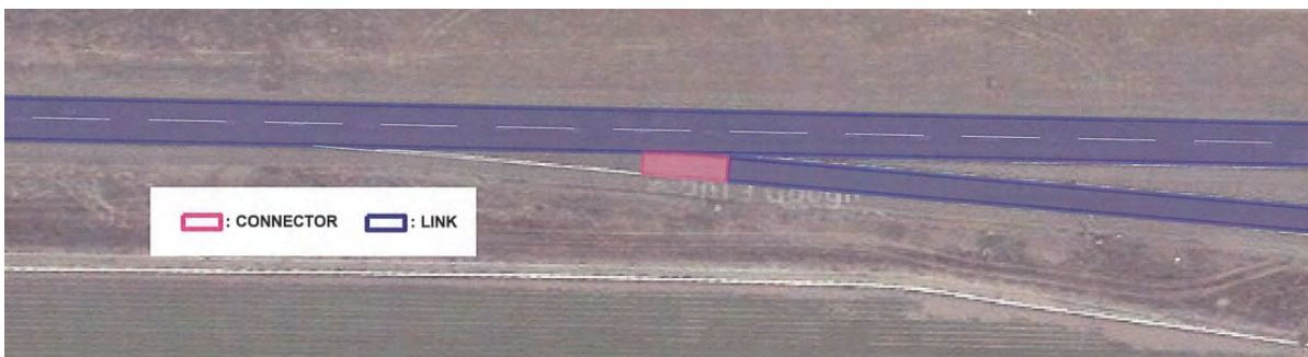
Figure 7 - Suggested Coding of a Freeway Diverge Area (taper)
