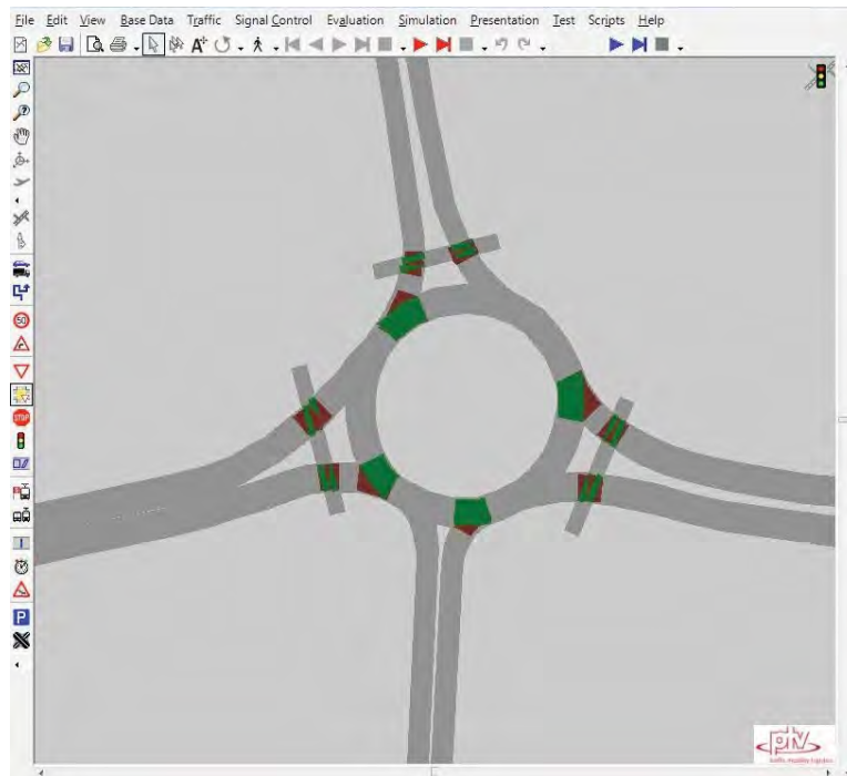
Figure 10 - Example Conflict Area at Roundabout
