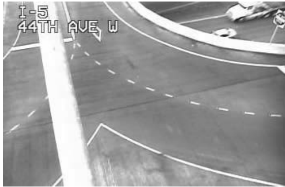
Guide striping provided for left-hand turns.
