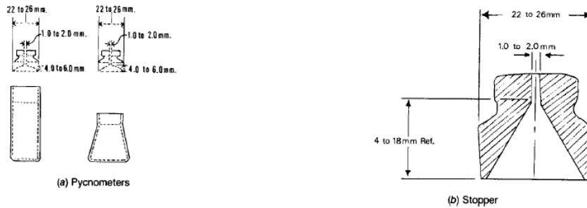
FIG. 1 Suitable Pycnometers and Stopper
