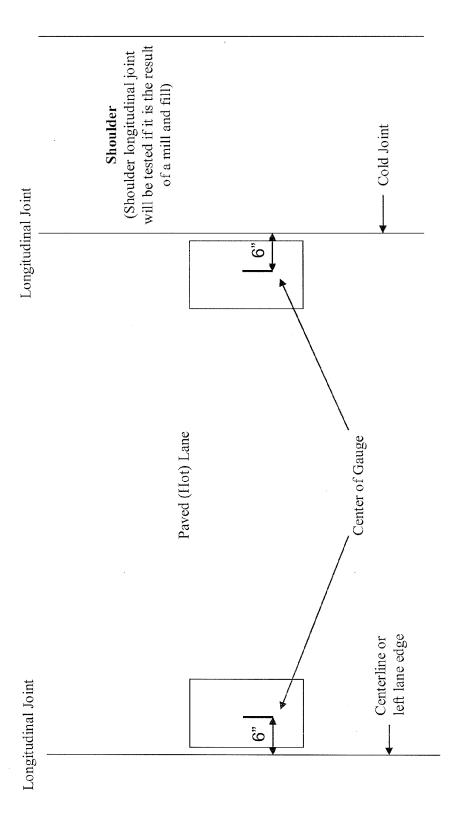
Longitudinal Joint Testing Locations *Figure 1*
