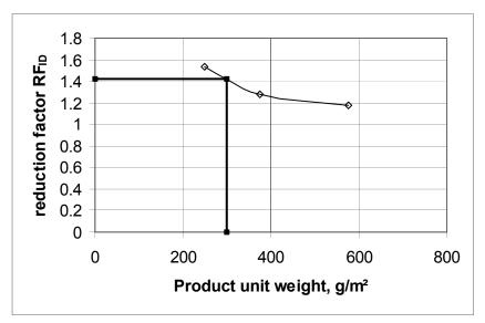
Figure, A-2. Example interpolation of  $RF_{ID}$  from damage measurements on products from the same line but with different weights. For a product of weight 300 g/m<sup>2</sup>, R  $F_{ID} = 1.42$  (Note: 1 oz/yd<sup>2</sup>= 0.0295 gm/m<sup>2</sup>).
