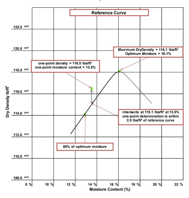
The results of a one-point determination were 116.5 lb/ft<sup>3</sup> at 13.5 percent moisture. The point was plotted on the reference curve graph. The one-point determination is within 2.0 lb/ft<sup>3</sup> of the point on the curve that corresponds with the moisture content.
