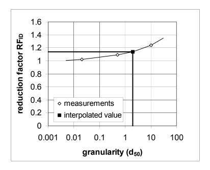
Figure A-1. Interpolation of RF<sub>ID</sub> for a soil with  $d_{50} = 2$  mm from installation damage data obtained for soils with  $d_{50} = 0.02$ , 0.5 and 10 mm (Note: 1in. = 0.0254 mm).
