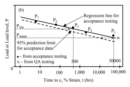
Figure 2. Conceptual illustration of the comparison of QA creep strain test results to initial product acceptance creep strain test results (a) creep strain curves, and (b) envelope of time to the specified strain.
