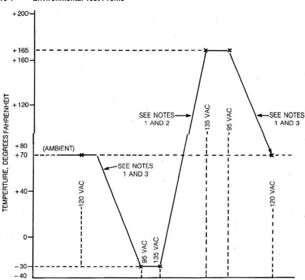
Figure 1 Environmental Test Profile
