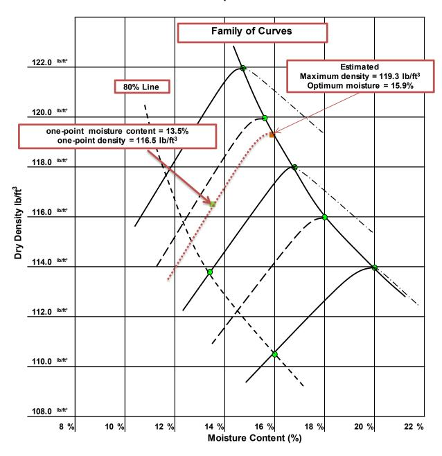
The results of a one-point determination were 116.5 lb/ft<sup>3</sup> at 13.5 percent moisture. The point was plotted on the reference curve graph. The point was plotted on the appropriate family between two previously developed curves near and intermediate curve.
