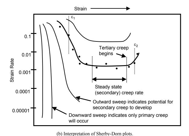
Figure C.1-2. Development and Use of Sherby-Dorn Plots to Analyze Creep Strain Data.
