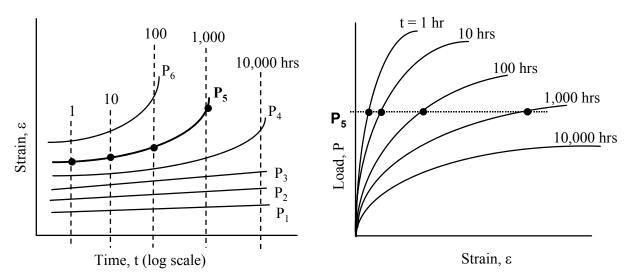
Figure C.1-4. Development of Isochronous Load-Strain Curves.
