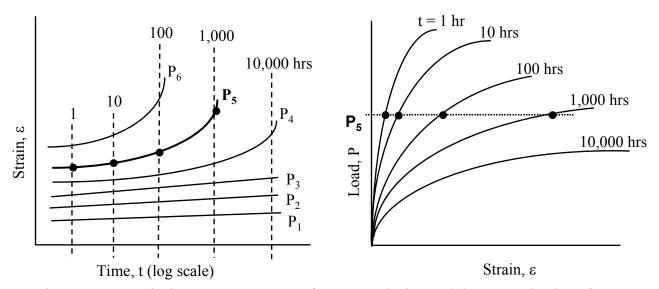
Figure B.2-1. Typical Stress Rupture Data for Geosynthetics, and the Determination of Shift Factors for Time-Temperature Superposition.
