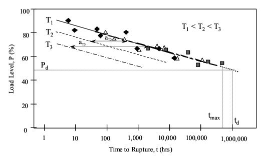
Figure B.2-2. Extrapolation of Stress Rupture Data and the Determination of the Creep Limit Load.
