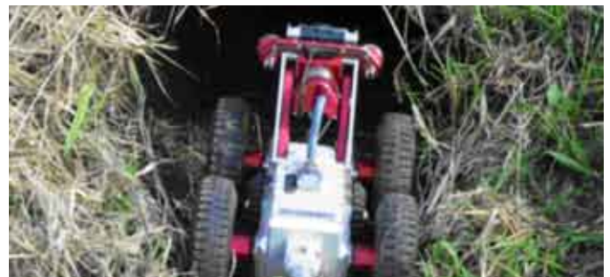
Meet Rover, the video culvert inspector
