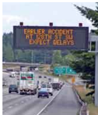
Variable Message Signs can give road conditions, warn of accidents and delays, and provide anticipated travel times.
