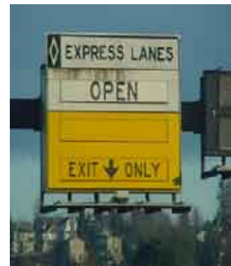
Changeable Message Signs have limited capabilities for communication. Generally they only provide the status, open or closed, of special lanes through a rolling drum.
