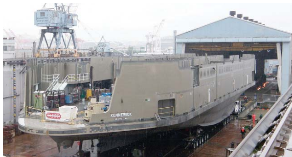
The MV Kennewick rolls out to dry dock from Todd Pacific Shipyards' main steel shop. The Kennewick will later be towed to Everett Shipyard for final outfitting and system testing.
