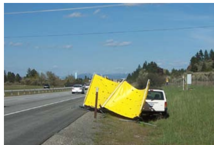
Portable screen is blown over from wind during April 27, 2006 test.
