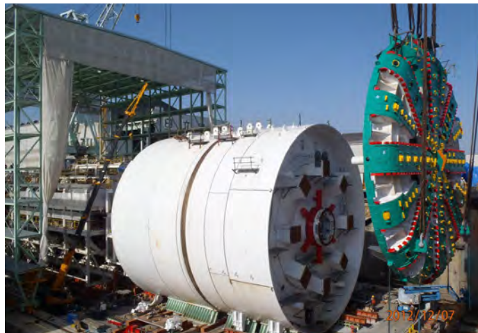
Giant cranes lift the 57.5-foot-diameter cutterhead into place on the SR 99 tunnel boring machine in Japan. Once complete, crews will test all components of the machine, including all motors, hydraulics, electrical and control systems. The machine is scheduled to arrive in Seattle from Japan in spring 2013, and start tunneling in summer 2013.
