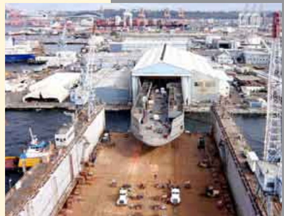
The Salish is moved from the Todd Pacific Shipyards construction hall to a dry dock via the level launch trestle.
