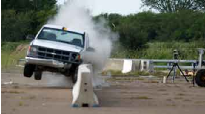
New guardrail designs are crash tested at the Texas Transportation Institute's crash test facility to ensure that new or modified roadside features are safe.
