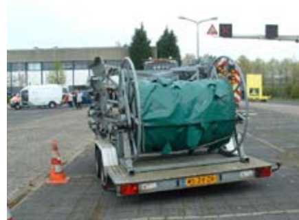
Portable screen on a trailer from the Netherlands. It can be up to 600 feet long and requires a 20-minute set-up by a trained crew.
