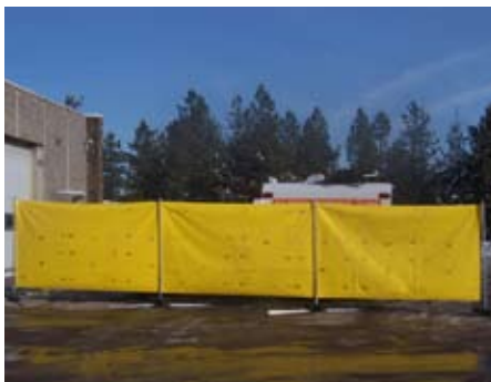
The top of a WSDOT Incident Response Truck peeks over one of the new Portable Incident Screens. Materials to build this unit cost about $500. The units are about 30 feet in length.
