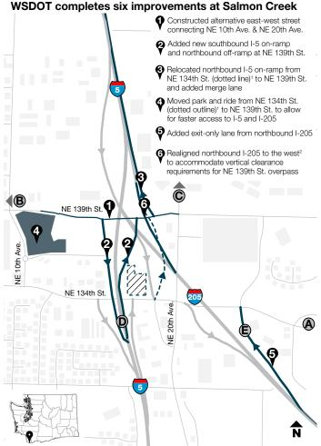
Notes: The dark lines represent the sections of roadway improved by the Salmon Creek project. Letter symbols are route origin and destination points. 1 Dotted lines are a ramp and park and ride that were moved as part of the project. 2 Realignment was too slight to see on map at this scale.
