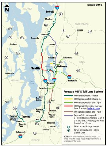
Approximately 244 lane-miles of a planned 369-mile freeway system of HOV-type lanes have been built in the Puget Sound region since 1970. In addition to the freeway mainline system, approximately 75 miles of transit or HOV lanes exist on state highway arterials and freeway ramps.
