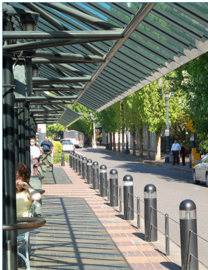
Cable, bollards and distinctive surfaces help define transit, auto and pedestrian areas.
