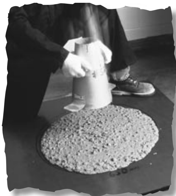
Left: Slump flow test. A technician lifts the slump cone and measures the diameter of SCC spread.
