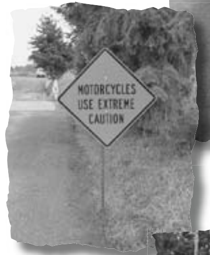
Temporary construction sign attached to a T-post.
