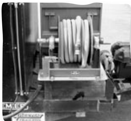
Hose reel for water supply.
