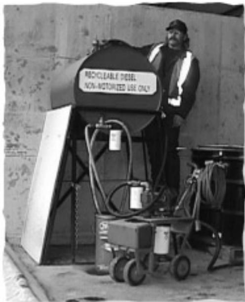
Patrick Zellner with Renton's Diesel Filtering Recycling System (Photo by Bill Wressel)
