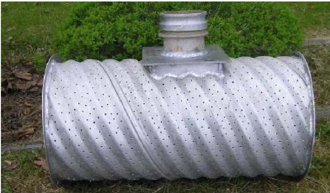
Figure 8. Example of a pump intake screen and pump outlet energy dissipater.
