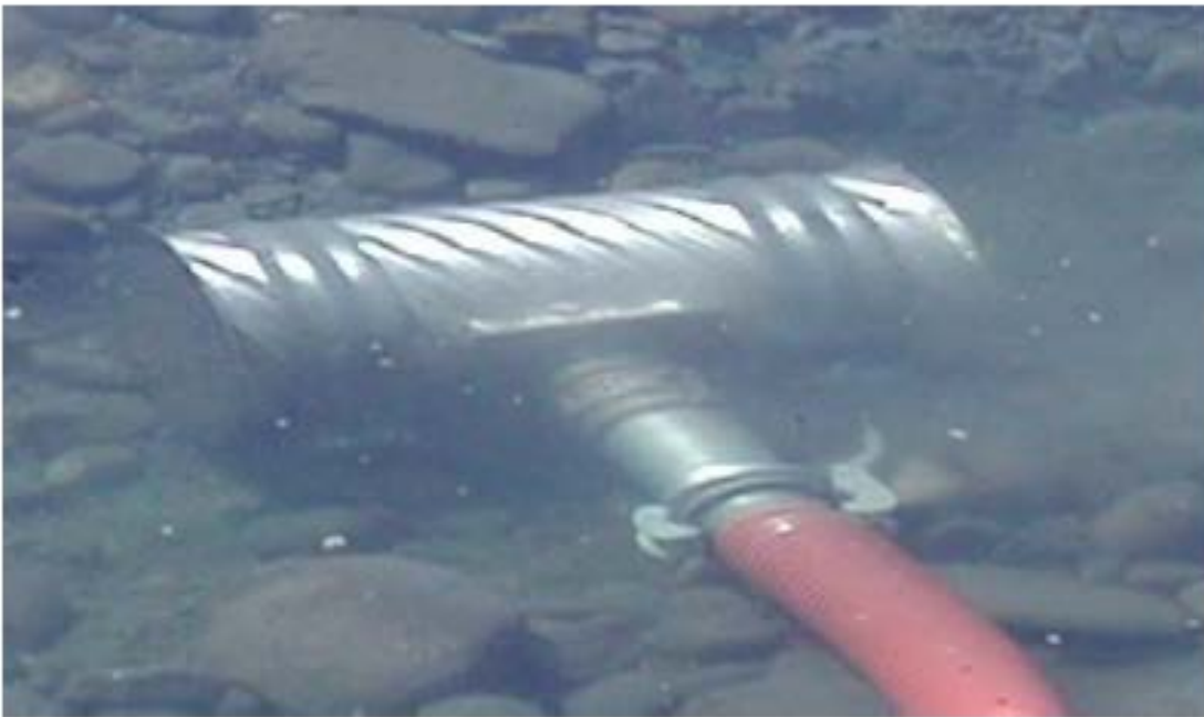
Figure 9: Pump Intake Screen.
